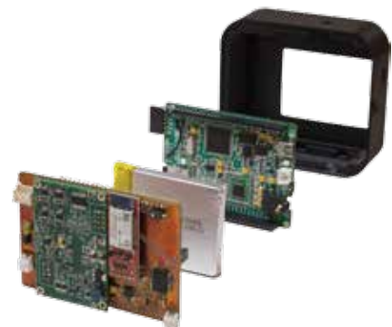
Exploded view of the microprocessor controlled rehabilitation device developed at NeuRA
